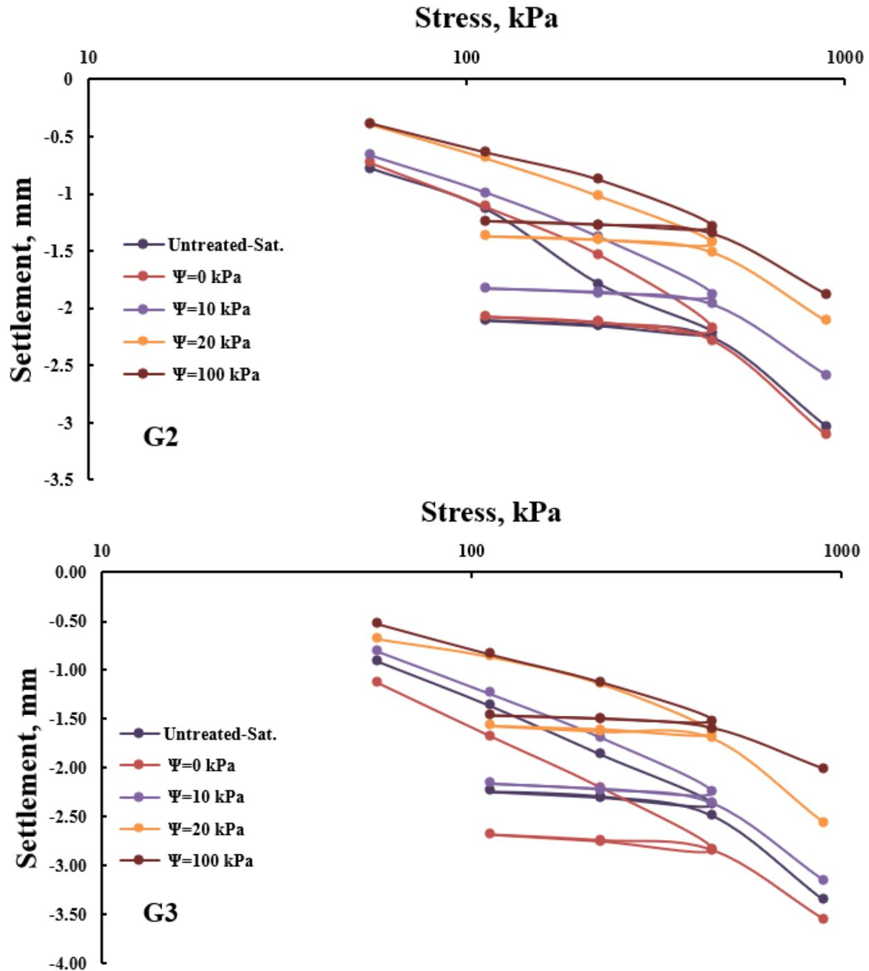
Figure 1. Load-settlement curves of 8.8%, 12.66%, and 30% of gypsum content for different stress conditions.
