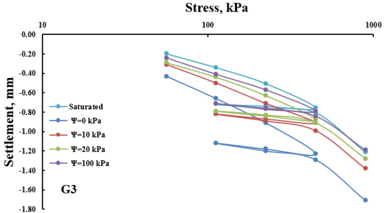
**Figure 2.** Load-settlement curves of 8.8%, 12.66%, and 30% of gypsum content for on the load-settlement behavior of Cement-treated soil
